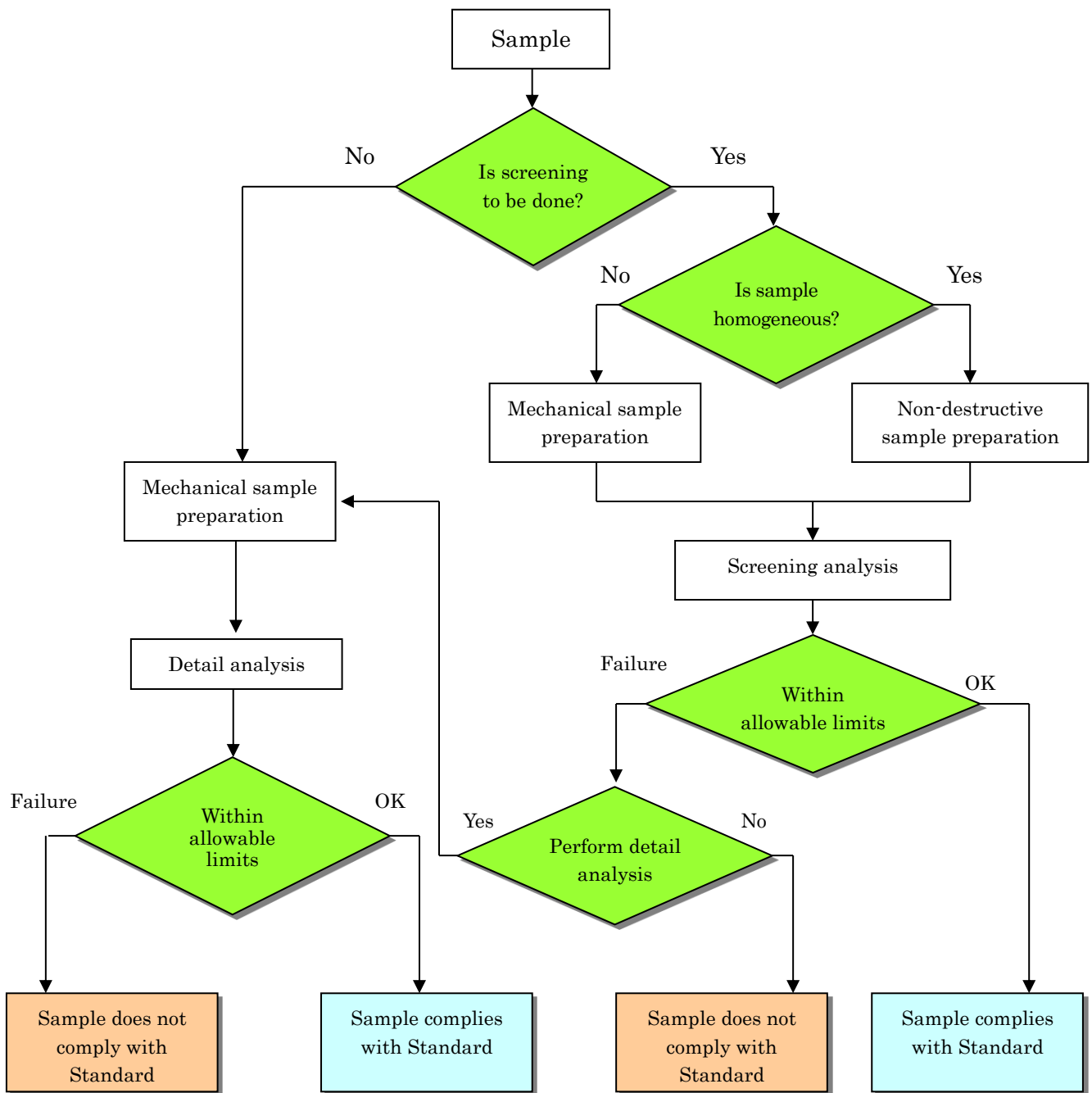
Fig. 4.28 Flow chart of analytical procedure
