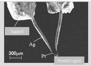
Electron microscopy image of the local heating mechanism
