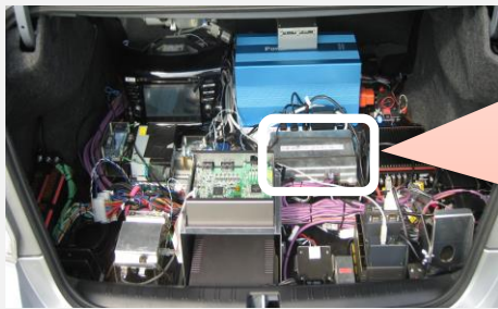
Autonomous driving system fits compactly into trunk
