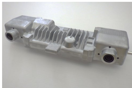
Stereo camera with nighttime pedestrian detection
