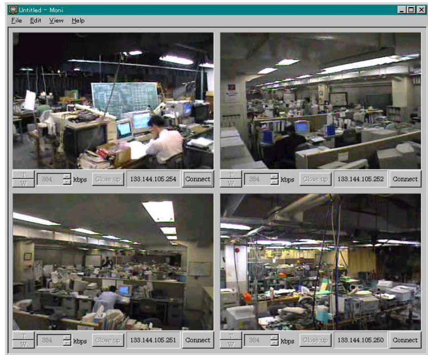
Fig. 2— Application Software Example. The screen lets the user select feed from a specific camera, control the actions of the camera itself, and change the amount of data transmitted.
