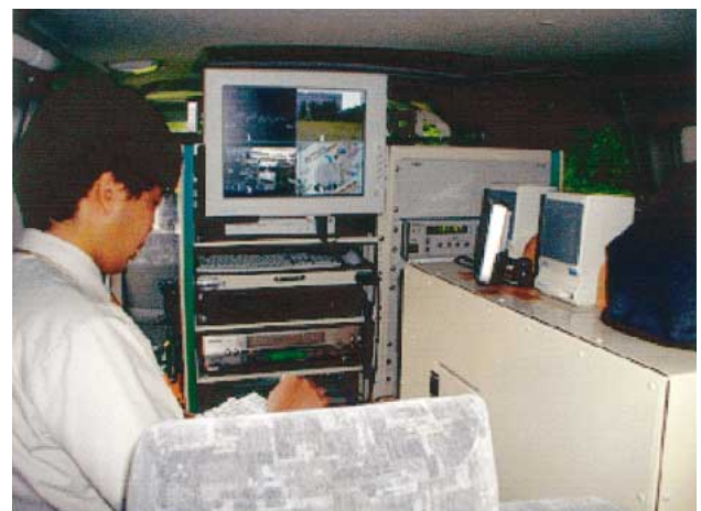
Fig. 5—Mobile Terminal Reception Experiment. Experiments on reception while the vehicle is traveling are being conducted with a terrestrial TV broadcasting receiver (center), evaluation equipment, a car navigation terminal (upper right) and other such devices installed in the vehicle.
