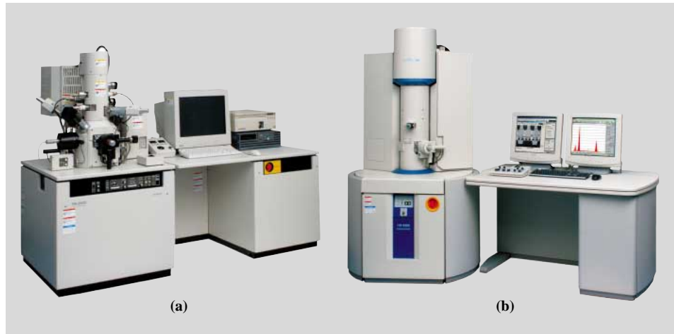
Fig. 1—Semiconductor Device Evaluation System is Composed of Focused Ion Beam System (a) and Ultra-thin Film Evaluation System (b). This evaluation system utilizes the 40-kV and the 200-kV accelerating voltages of the focused ion beam system and the ultra-thin film evaluation system, respectively, and it completes failure analyses of semiconductor devices and structure analyses of sub-nanometer areas within a few hours.
