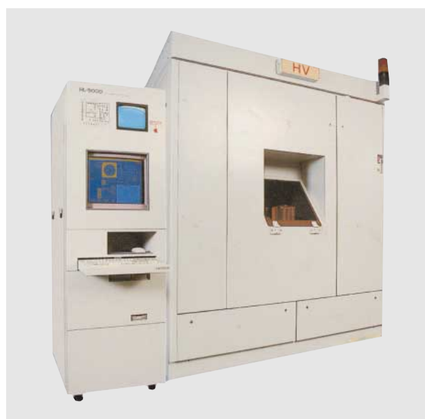
Fig. 1—Appearance of EB Lithography System. To attain high-precision writing, the apparatus's main unit and the control circuits to be controlled precisely are housed in a temperature-controlled chamber.
