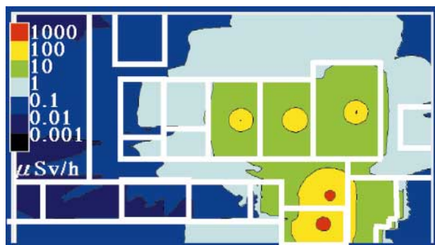
Fig. 4—Radiation Exposure Distribution in PET Facility Caused by Radiation from Patients. Amount of radiation exposure in the facility from the patients was simulated and evaluated.
