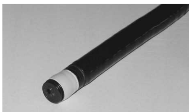
Fig. 10—External View of Electronic Radial Ultrasound Endoscope.
