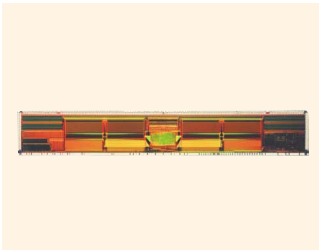
The HD66777 chip for implementing dual TFT liquid crystal display systems measures 19.97 × 3.17 mm.
