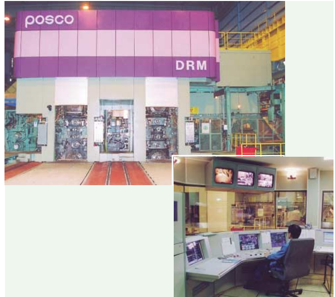
DCR steel rolling equipment at POSCO, and operating room with single operator (bottom right)
