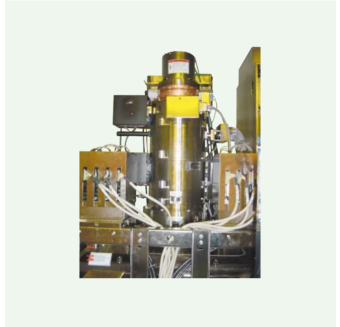
General view of electron beam mask writer: HL-7000M
