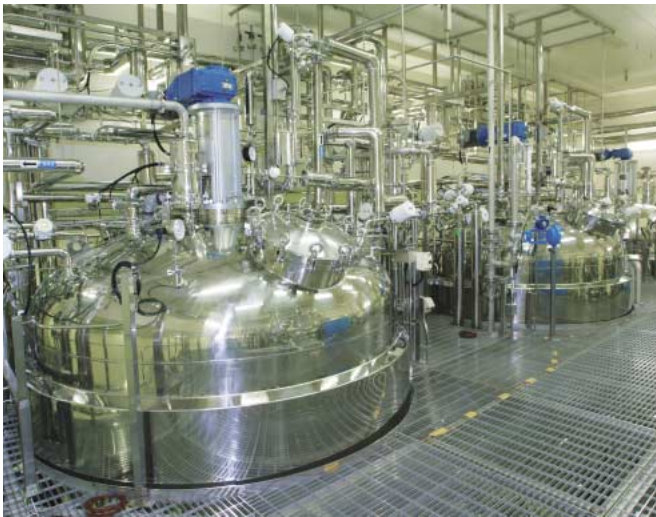
External view of scaled-up main cell culture reactors
