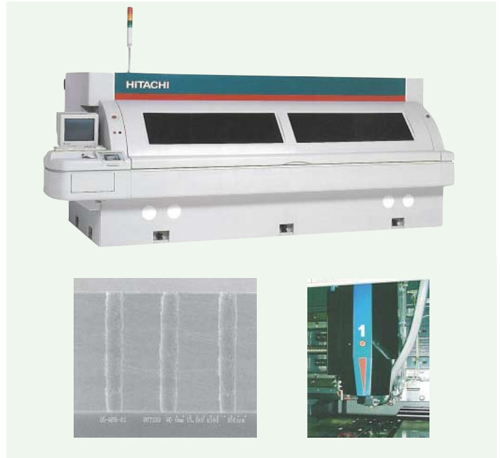
ND-Q series drilling machine with 300,000-min -1 spindles (top), 50-µm via-hole section view (bottom left) and direct-drive z-axis (bottom right)
