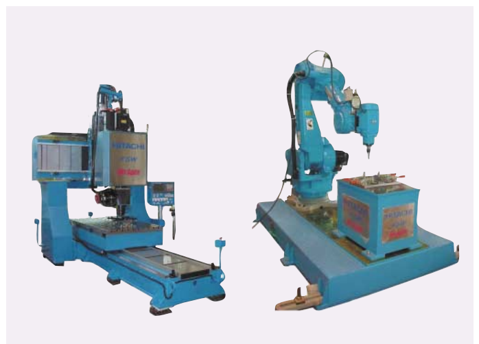
(c) 3-D FSW machine (left) and FSW robot (right)
