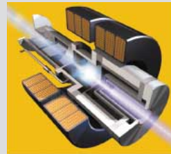
(b) Microwave ion source
