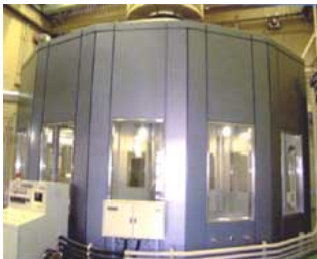
Fig. 10— The Sodium Fire Experimental and Extinguishment Equipment Is Used for Observation of Sodium Combustion and Training in Using the Special Fire Extinguisher (photo from JNC).
