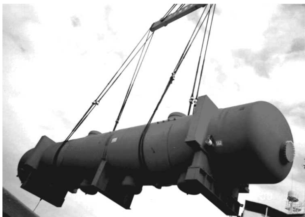
Fig. 3— Improved-Type MSR. The overall length could be reduced by increasing the steam flow velocity and separating the drain tank from the MSR.
