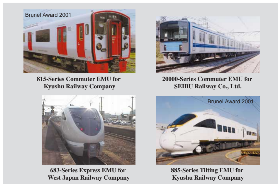
Fig. 1— The “A-train” Family of Trains. To meet the requirements for various types of rolling stock, a next-generation, aluminum carbody system—which incorporates several new concepts and ideas—called the “A-train” structure is being developed.
