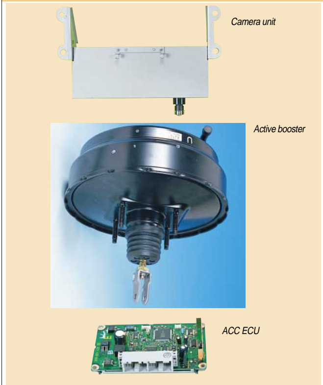
Adaptive cruise control (ACC) system
