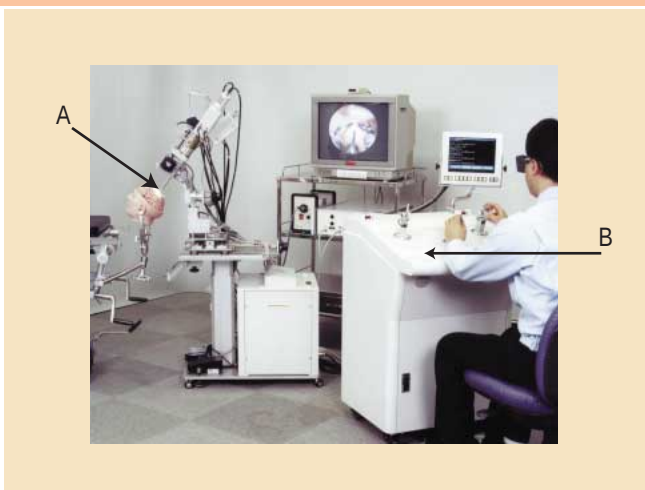
Prototype system supporting minimally invasive neurosurgery In a thin insertion probe, [A] three micro manipulators are bundled together; a surgeon is operating from an operating console [B]
