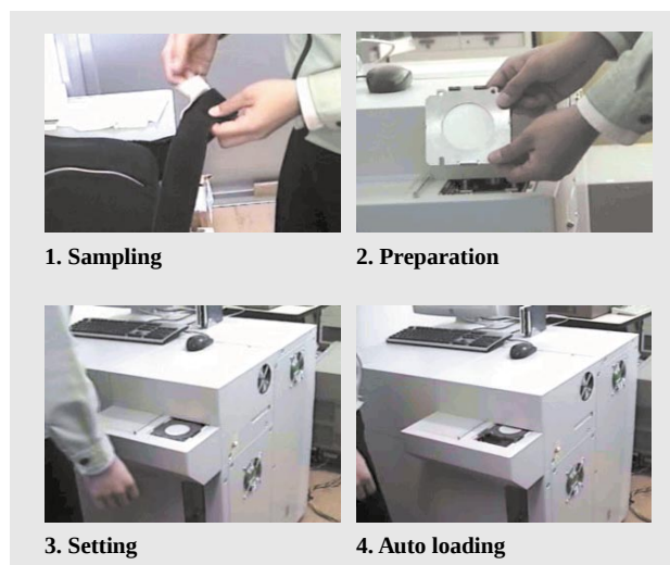
Fig. 4—Operation Procedure for Drug-trace Detection. Once the wipe material is set in the predetermined place, measurement is performed automatically.
