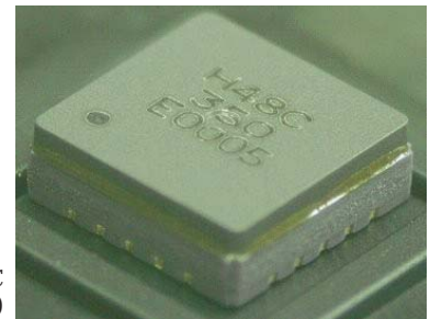
New accelerometer: H48C (4.8 mm 2 × 1.5 mm thick)
