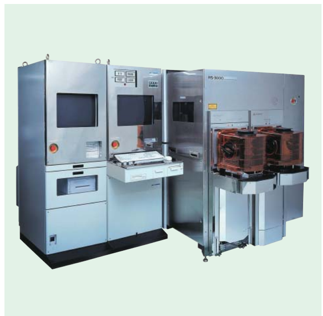
RS-3000 V5 in-line defect review SEM
