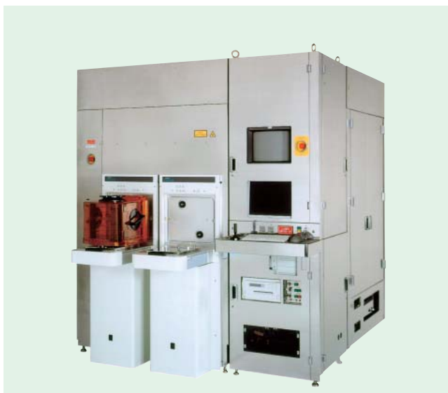
Highly sensitive, high-speed, dark-field wafer-inspection system: IS2700E
