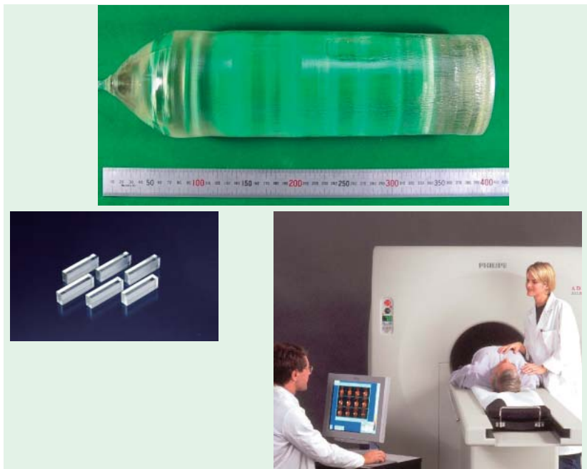
Large GSO single crystal with size of \phi 105 \times 290 (mm) (above), GSO-PET "ALLEGRO" (below right) and GSO scintillators (below left)
