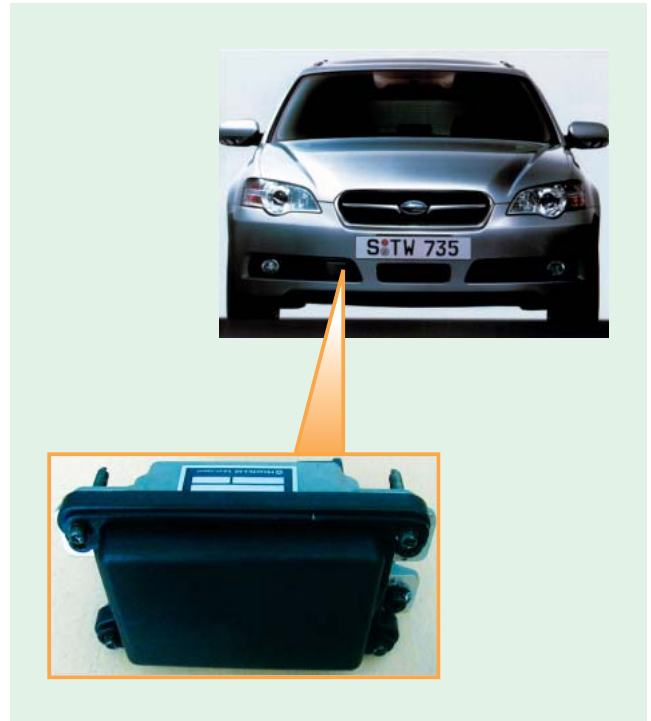
Subaru Legacy Touring Wagon 3.0R with ADA system (above) and Hitachi millimeter-wave radar (below)
