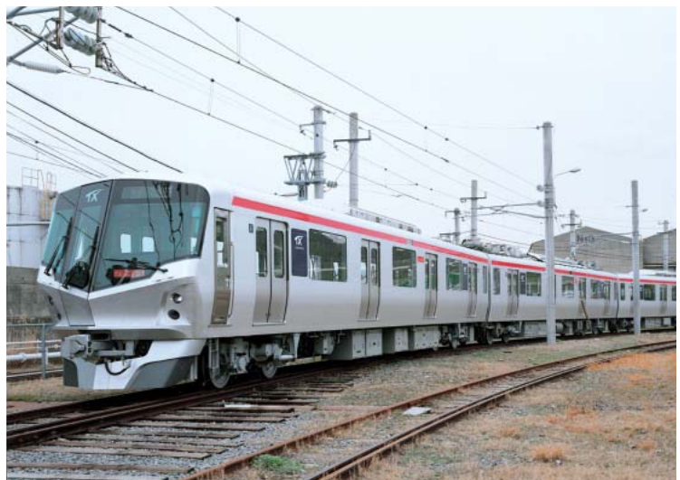
Tsukuba Express dual-voltage AC/DC electric trains
