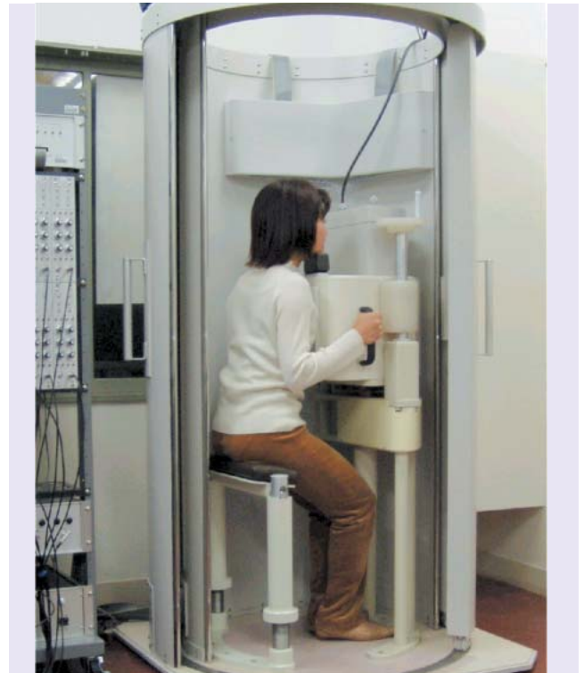
Mobile and space-saving high-temperature superconducting magnetocardiograph system for heart disease screening tests
