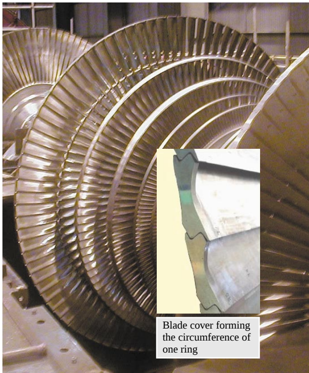
Fig. 4—External View of Low-pressure Rotor Utilizing CCBs for All Blade Stages.
