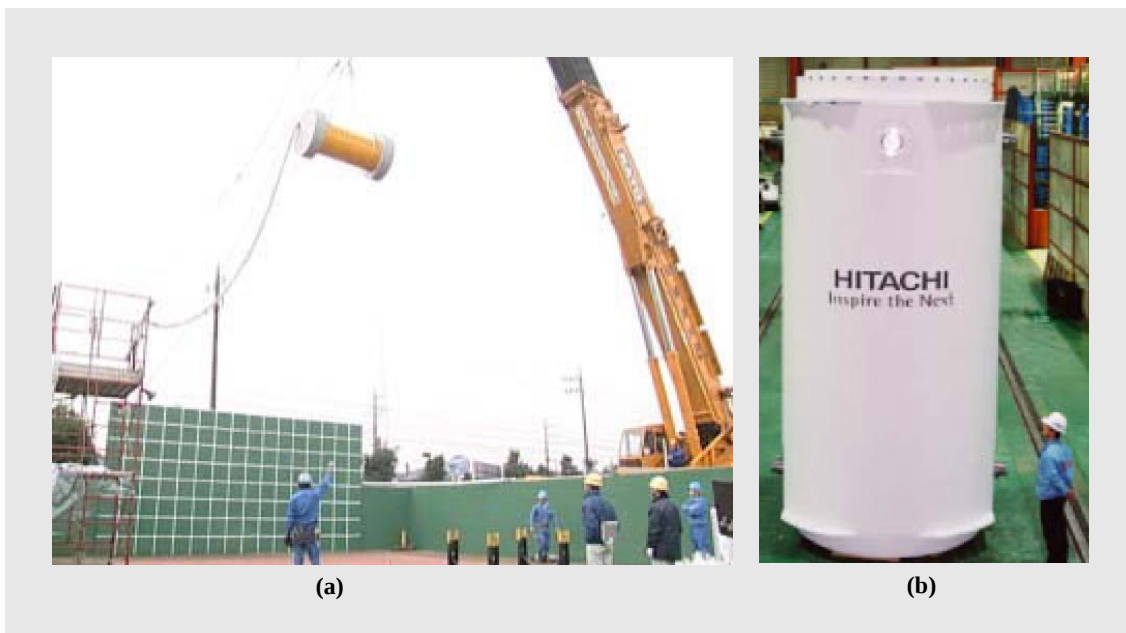
Fig. 1—1/3 Scale-model Drop Test (a) and External View of 1/1 Scale-model (b).
