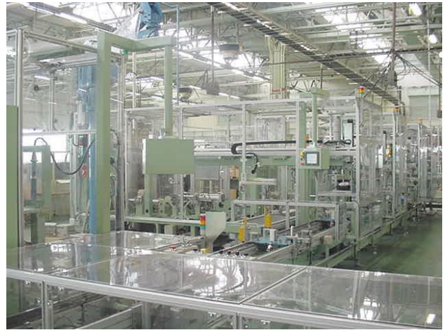
Fig. 6—Motor Assembly Line for HEVs. Production capacity is 5,000 units per month.
