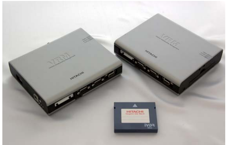
Prototype of VRM terminal with interfaces to GPS, HDD, PCMCIA (Personal Computer Memory Card International Association), wireless LAN, and in-vehicle LAN
