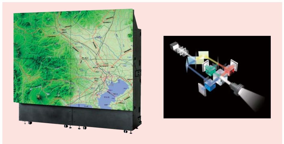
70-inch 2 × 2 LCOS video wall (left) and LCOS optical engine (right)
