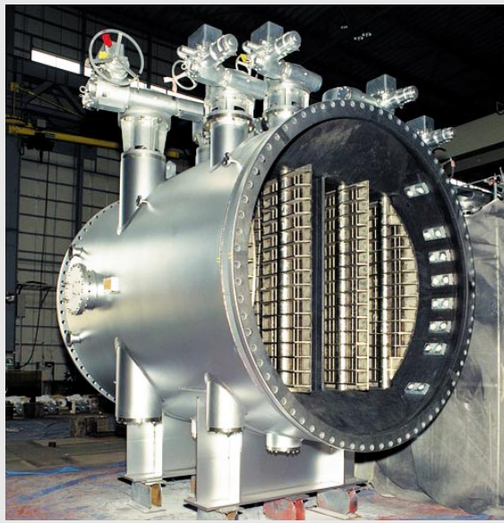
(a) Ball strainer with flapping screen (shell diameter: \phi 3,500 mm)
