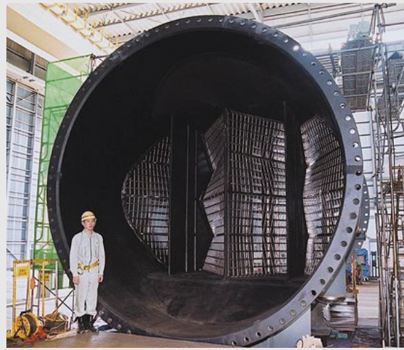
(b) Large-capacity ball strainer (shell diameter: \phi 4,400 mm)
