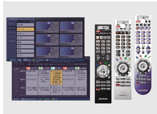
Fig. 6—Product Prototypes Assessed by Consumers. Prototypes of proposed products are given to consumers (including elderly and handicapped users) to try out, and their assessments are reflected in the final product specifications.
