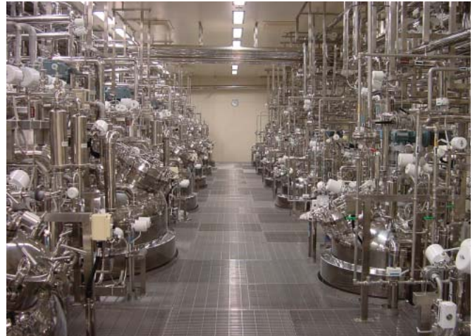
World's largest class mammalian cell culture plant: six 10,000-L scale mammalian cell culture reactors
