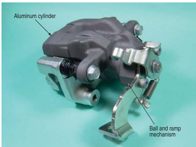
Aluminum rear caliper for high gas mileage and utility
