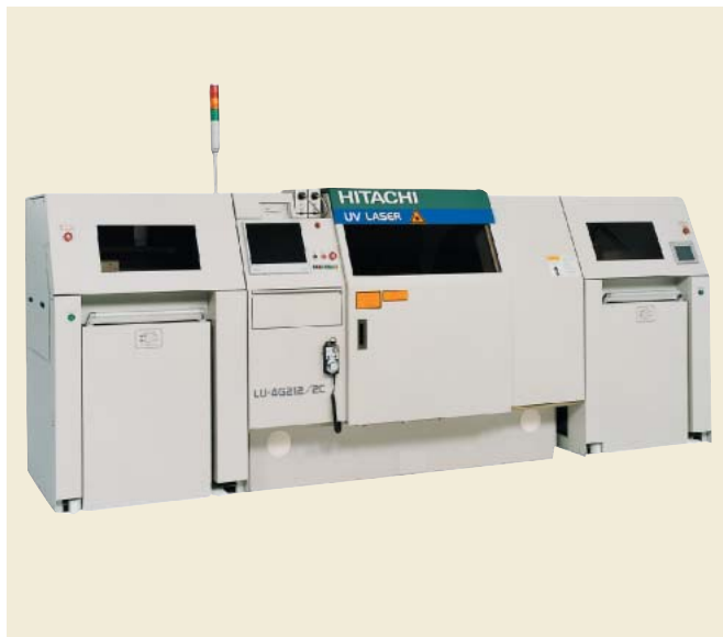
Four-beam UV laser drilling machine, LU-4G212, that drills two panels simultaneously using four beams scanned by 2,000-hole/s galvanometer scanners
