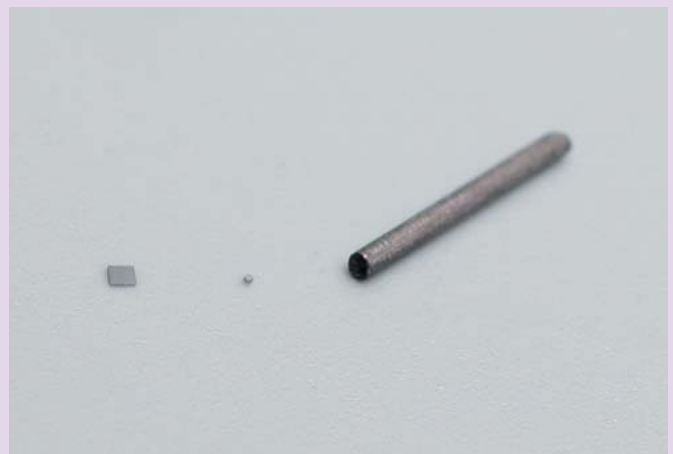
The current chip (left), the newly developed chip (middle), and a mechanical pencil lead (right). Newly developed chip is 0.15 mm per side and 7.5- \mu m thick. The new chip occupies only one-seventh of the area and one-eighth of the thickness of the current model, which measures 0.4 mm per side and is 60- \mu m thick.
