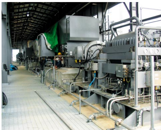
Fig. 5—5,800-kW Motor-driven Gas Compressor. Photo of sales gas compressor installed at the Betara Gas Processing Plant.
