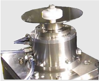
Fig. 13—Spindle Motor. The motor has a static-pressure air bearing with rotation non-repeated fluctuation at the sub-nanometer level.
