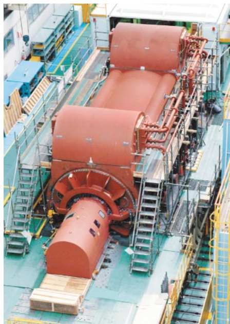
Fig. 1—Completed 1,120-MVA 50-Hz Generator at the Manufacturing Plant (Left), and Stator Frame Being Moved by Crane at the Manufacturing Plant Prior to Delivery (Right). Reliability and design are closely evaluated at the manufacturing plant through rotational tests and a host of other tests and evaluations.
