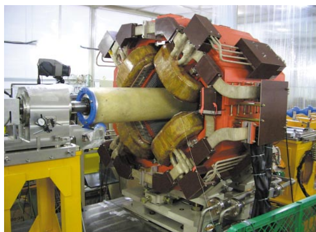
Fig. 3—3-GeV Quadrupole Magnet during Magnetic-field Measurement.
