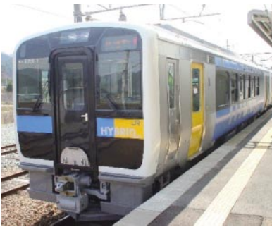
Fig. 4—JR East’s Kiha E200 Series Diesel Railcars. The Li-ion battery assisted hybrid drive system was developed in collaboration with JR East.
