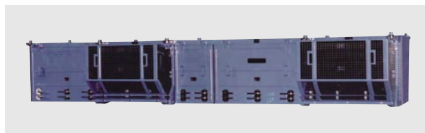
Fig. 3—External View of VVVF Inverter. The inverter is configured as a “longitudinal-box construction” so it can be handled from the side of the car body.
