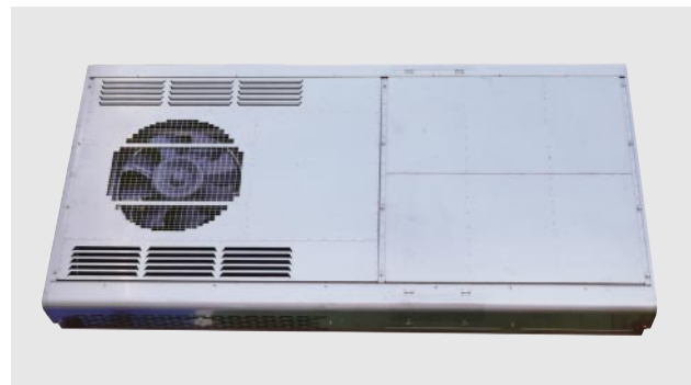
Fig. 8—External Appearance of Air-conditioning Unit. Since the unit is fitted within the boundary of the train car, a low-profile air-conditioning unit could be adopted.
