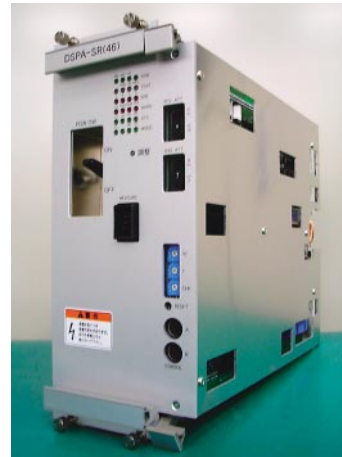
Fig. 3—DSP/PA Transceiver Unit. Integrating the DSP and PA saved space by increasing the implementation density of the transceiver unit.
