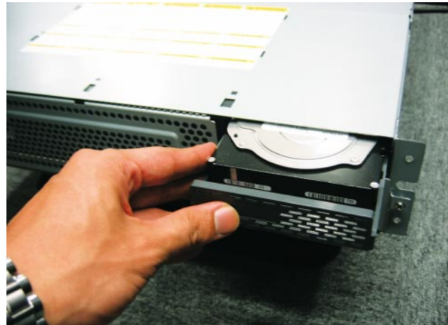
Fig. 4—Inserting an HDD into a Repair Slot.
