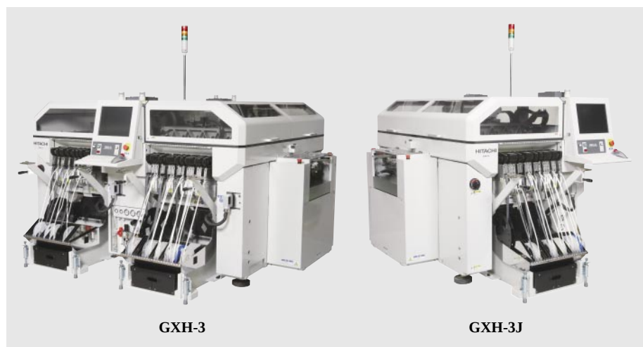
Fig. 1—Photos of Modular Direct Drive Mounters GXH-3 and GXH-3J. Hitachi's latest modular direct drive mounters are fast, accurate, provide excellent placement accuracy, achieve a throughput about 20% better than previous placement equipment, and are now commercially available. GXH-3 on the left has a throughput of 95,000 chips per hour, and GXH-3J on the right has a throughput of 47,500 chips per hour.
