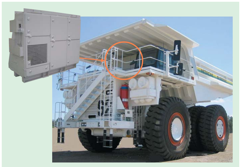
Dump truck for mines and control cabinet containing the inverter (left top)
