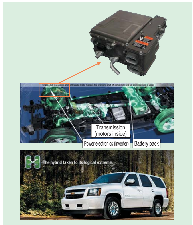
"TPIM" inverter and GM Tahoe with the TPIM
