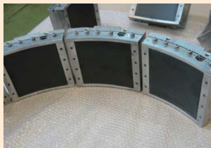
Bearing assembly (upper) and bearing surface (PPS) (lower)
