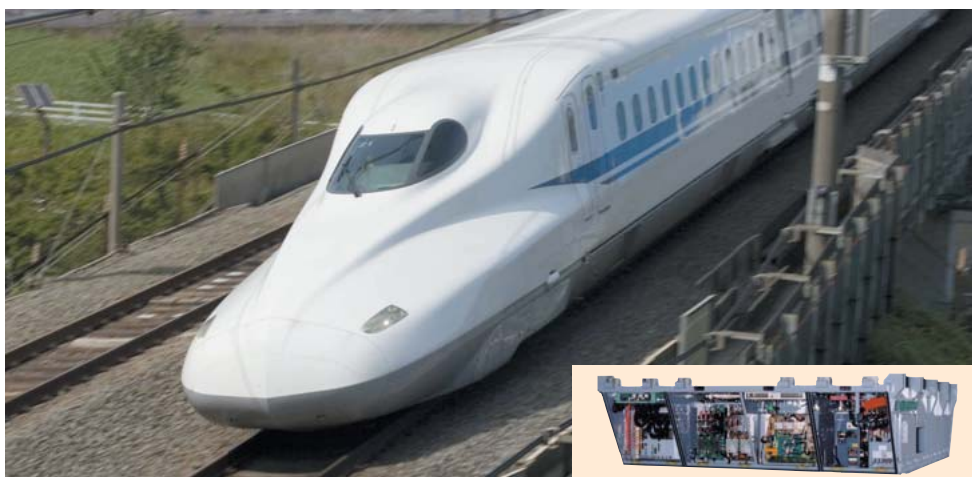
N700 Shinkansen car (above) and its main converter (right)
