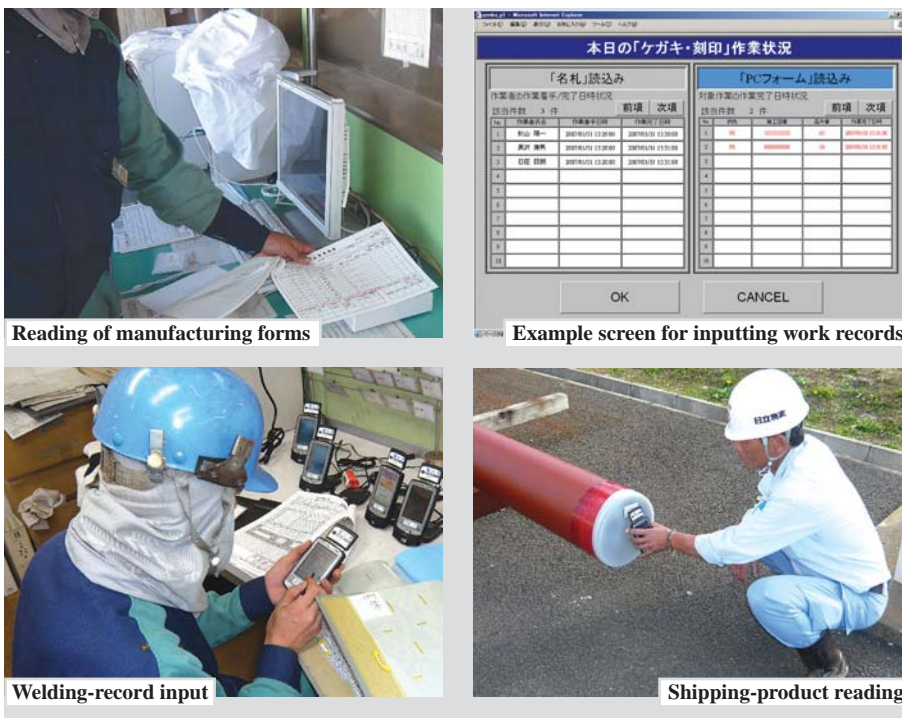
Fig. 3—Examples of Scenes of Workers Using RFID Technology and a Work Input Screen at Pipe-production Plant. RFID technology is applied to work-record collection and welding control as well as shipment control of piping.
