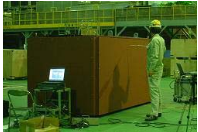
Fig. 10—External Scene of Noise Testing with a Mock-up Model.
