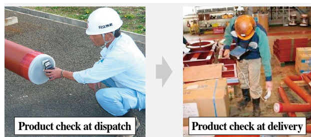
Fig. 7—Use of RFID with Products and Materials. RFID is used for product identification and data input at dispatch and delivery.
