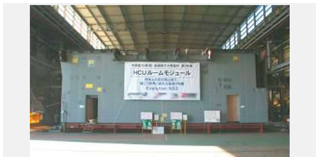
Fig. 3—HCU Room Module. The entire HCU (hydraulic control unit) room module at the dedicated module factory prior to shipment is shown.
