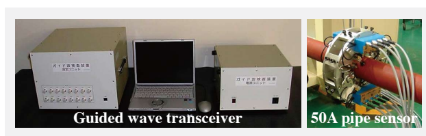
Fig. 9—Portable Guided Wave Inspection System.
