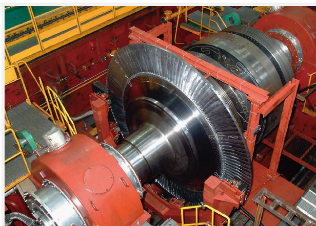
Fig. 5—Full-scale Operating Model Test Facility. Vibrational characteristics can be verified under the same vibrational force conditions to which the actual turbine is subjected.
