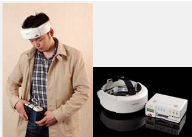
Fig. 5—Wearable OT. Experimentally developed wearable OT system weighs only 1 kg (400 g for the measurement unit).
