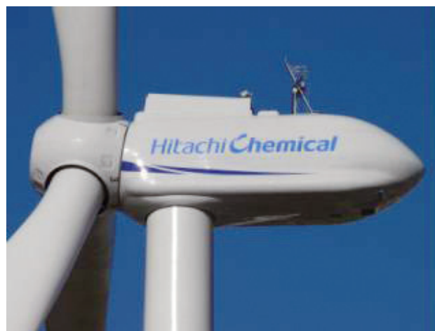
Fig. 4—Nacelle of 2-MW Downwind Turbine.
