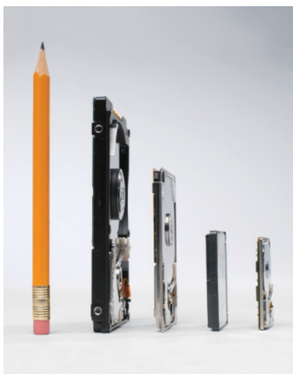
A lineup of Hitachi HDDs (from left: 2.5 inch, 1.8 inch, 1.0 inch and 1.0 inch (planned))
